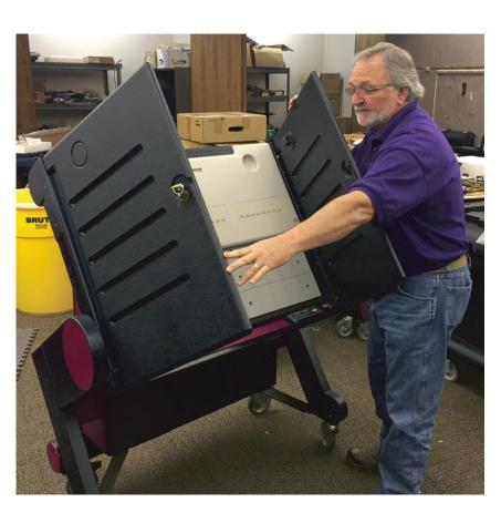
Lower the voter panel to the DOWN position. Do this by pulling the **maroon** latch release. DO NOT FORCE THE VOTER PANEL DOWN!
